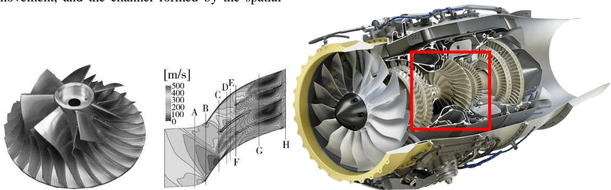
(a) Centrifugal compressor with double splitter blades and its simulation results [9] (left). (b) HF120 engine/manufacturer GE Honda Aero Engines (GHAE) (right).
