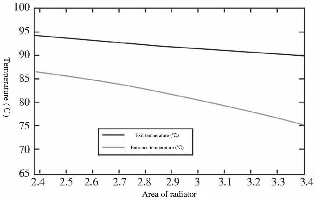
Figure 8 Effect of the windward area of radiator on heat dissipation performance [6].
